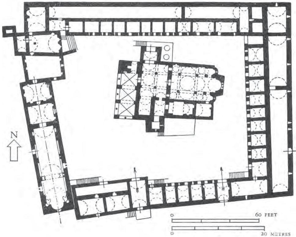
Figure 10.1 Plan of the monastery of Osios Meletios on Mt. Kithairon in central Greece. Byzantine monasteries normally took the shape shown here: a rough rectangle that served as a defensive wall and the location of the rooms that comprised the cells of the monks. A formal reception room and the quarters of the abbot would also normally be located in the exterior circuit. The interior of the enclosure would be dominated by the church, or, often by two churches: one reserved for the monks and the other open to visitors as well. The monastery would also include a kitchen and bakery, along with a dining room ( trapeza ). The latter commonly was a separate building that often was elaborately decorated, although at Osios Meletios these facilities were built in to the exterior.
